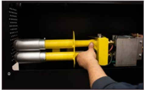
6 - - Remove the burner from the compartment
